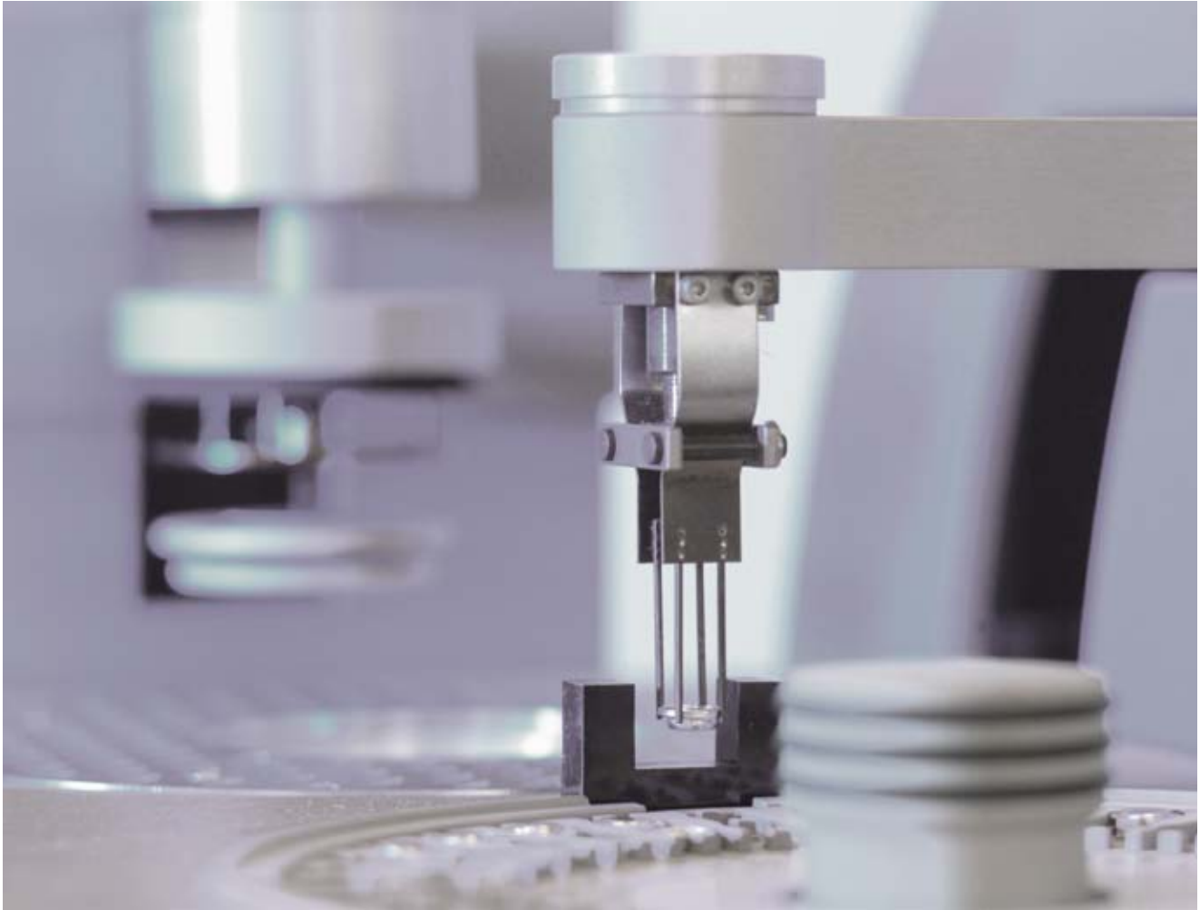
Incoming inspection: Differential Scanning Calorimetry (DSC). thermal analysis of materials.
