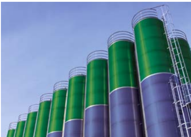
Secured raw-material supply and batch tracing by means of dual-chamber silos.
